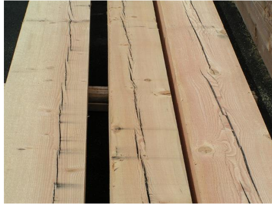
Grieta longitudinal Foto: https://www.carolinatimberworks.com/why-do-timbers-split-and-crack/
